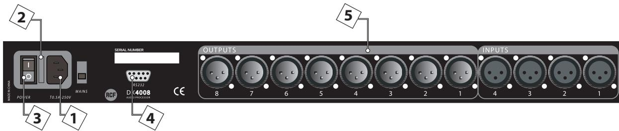
**1. Main Power** - Connects via a standard IEC socket. A compatible power cord is supplied with the unit. The voltage input is either 115VAC or 230VAC and is clearly specified on the unit. Voltage requirement has to be stated upon ordering.
