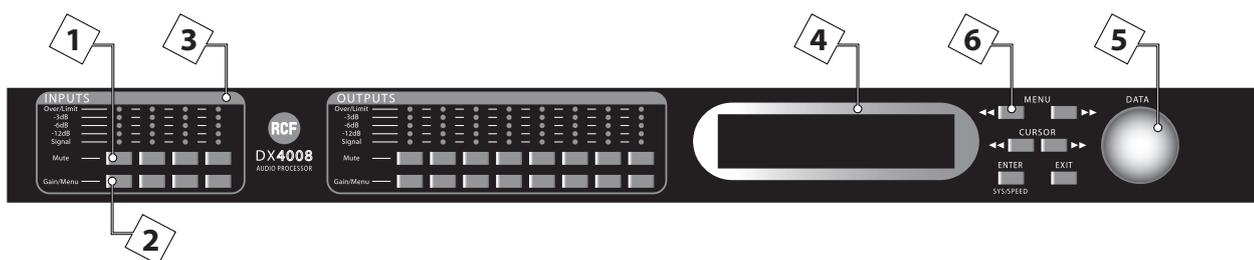
**1. Mute keys** - Mute/Unmute input and output channels. When an input channel is muted, a red LED will be lit for indication.
